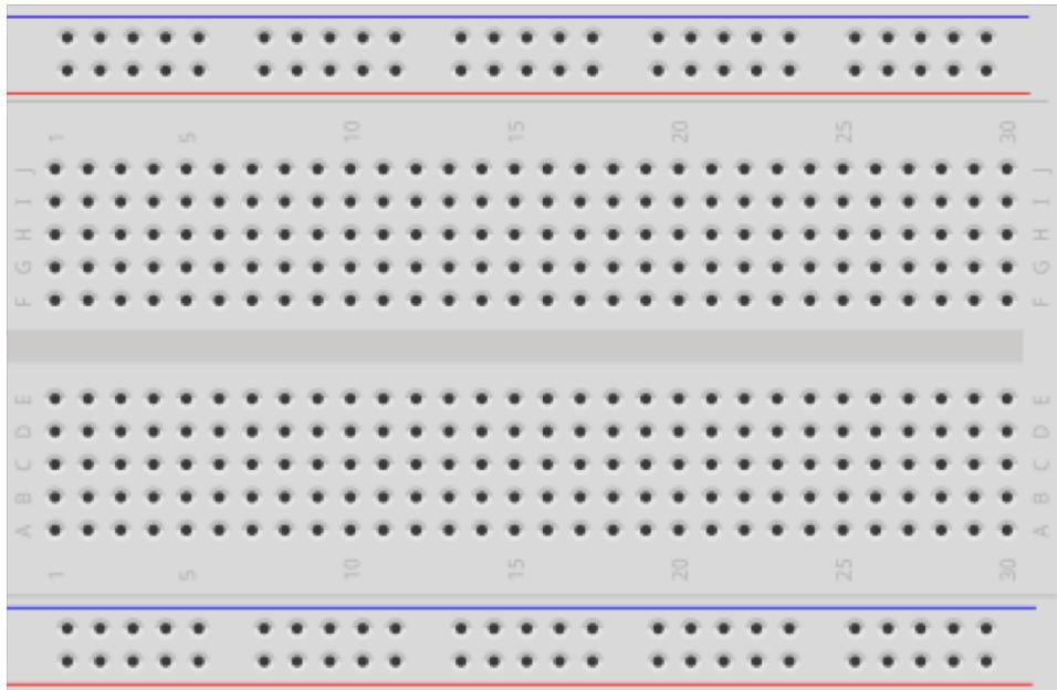
A breadboard is used to wire electric components together
